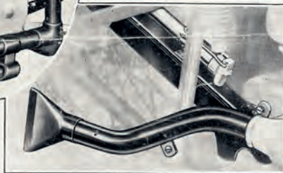
BELOW: Close up of the new enlarged Parkerized tail pipe with new fish-tail silencer.
