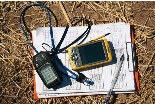
Fig. 3, 13 PDA Trimble Juno SB, GPS Garmin eTrex and the paper documentation. Photo by Tereza Včelícová.
